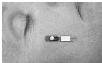
OneDosePlus TM self-adhesive dosimeter with integrated build-up
