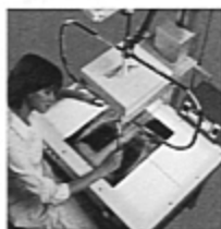
Treatment areas are easily traced with a free-moving stylus. A rigid, heated cutting wire follows the traced pattern for a clean block cut.
