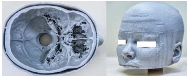
Figure 1. The 3D-printed patient specific hollow phantom before gel filling and phantom sealing. High 3D-printing accuracy of bone structures was implemented.
