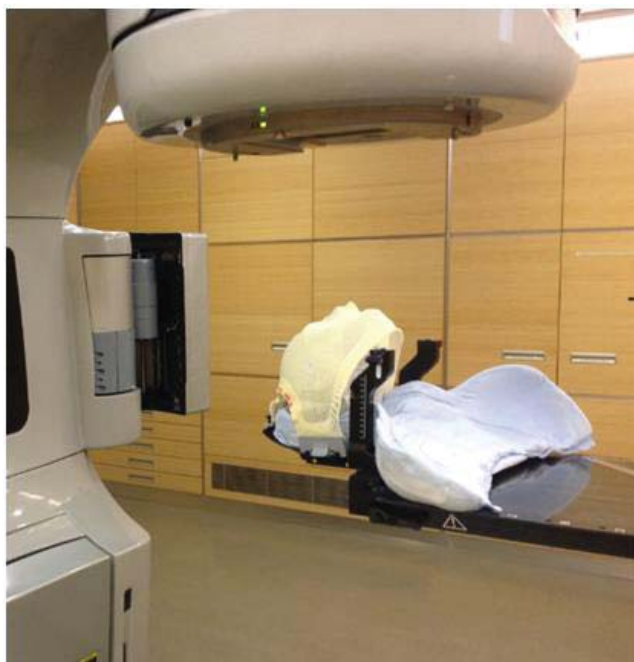
Figure 2. Set-up and Image Guidance of the PSDP as if it is the real patient.
