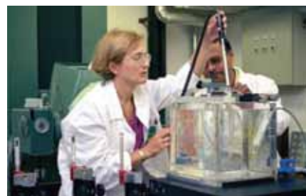
Calibration of an ionization chamber at the IAEA Dosimetry Laboratory
