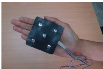
Fig.1: Palm worn electrodes to measure respiration rate of a baby without making it cry, for use with FIM system.
