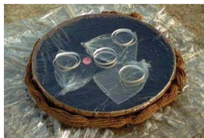
Fig.2: Very low cost solar water pasteurisation device for rural homes. It uses easily available materials.
