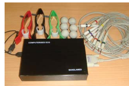
Fig.3: 12 lead digital ECG for use with telemedicine, or as a stand-alone equipment.
