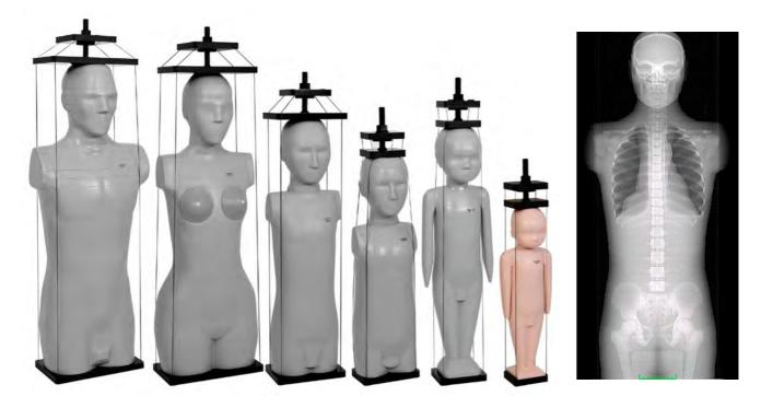
**ATOM**<sup>®</sup> **Phantoms** provide accurate simulation for both diagnostic and therapeutic energies while an organ dosimetry feature optimizes detector placement for precise calculations during whole body and organ dose mapping studies. Only ATOM offers a full range of ages: newborn, 1-year old, 5-year old, 10-year old as well as the adult male and female phantoms. These sizes ensure simulation of appropriate dose based on the size of your patient.
